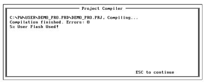
The amount of memory used in the user bank (FlashPROM in the Panel) is also shown after a successful compilation. See the *PANELWARE*<sup>TM</sup> *Hardware Installation User's Manual* (GFK-0848) for more information.
